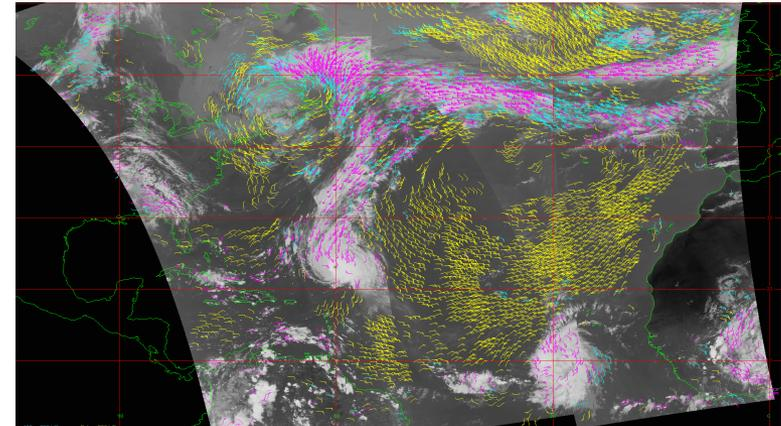
An example of low-latitude coverage over the northern hemisphere Atlantic Ocean of VIIRS IR winds from alternating passes from S-NPP/NOAA-20, color-coded by height: Yellow ( $> 700$  hPa), cyan (400 - 700 hPa), magenta ( $< 400$  hPa).
