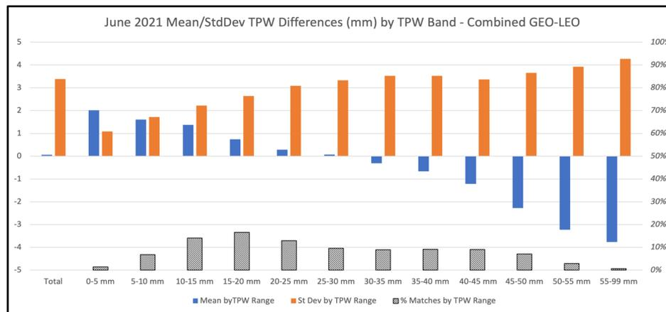
Errors in TPW vs. surface GPS/TPW measurements for combined GEO/LEO analysis before bias correction
