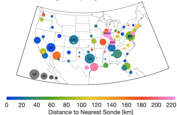
Locations of aircraft-based profiles of temperature and water vapor. Size of dot corresponds to average number of daily profiles while color represents the distance to nearest radiosonde launch site.
