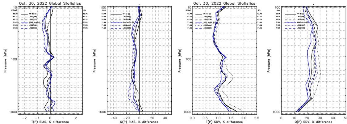
Temperature and moisture bias (left) and standard deviation (right). Coupled physical retrieval is plotted in solid line. Regression trained on cloudy radiances [REG(cldy)] is plotted as dotted line. Regression trained on cloud clear radiances [REG(CCR)] is plotted as dashed line. NOAA-20 statistics in blue on 30 Oct 2022 was included for comparison.
