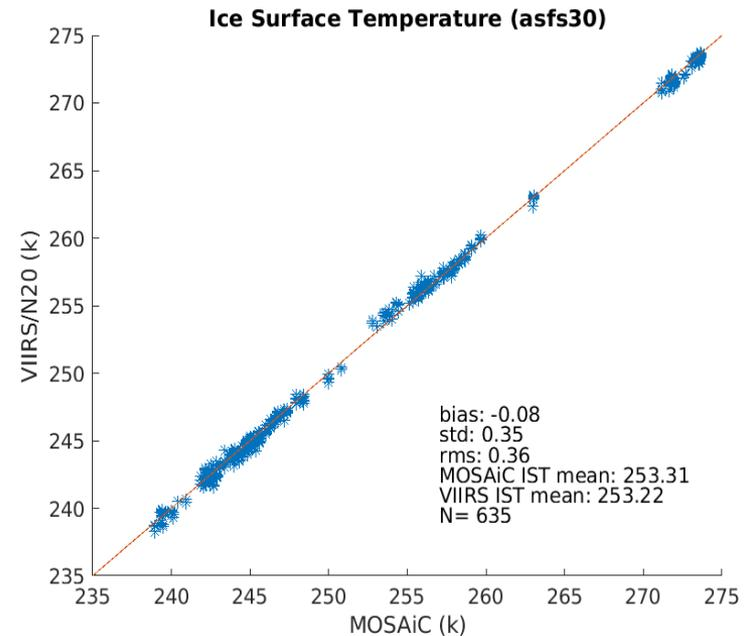
Ice Surface Temperatures (IST) under clear sky condition from NOAA-20 VIIRS compared to MOSAiC data, during November 2019 through July 2020 period over central Arctic north of Svaalbard.
