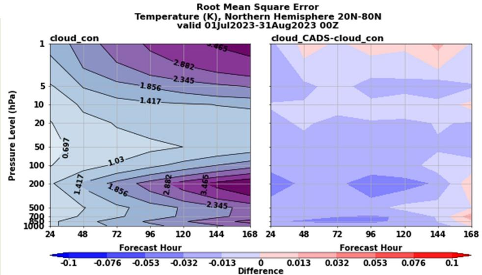
The left panel indicates the temperature forecast error growth within the model from 24 to 168 hours of the control (cloud\_con). The right panel is the **change** in temperature error growth when using the new cloud detection scheme (cloud\_CADS – cloud\_con). The varying shades of blue indicate improvements (less error) in the temperature forecast when using the new cloud detection scheme.
