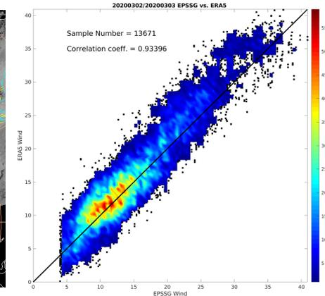
ERA5 vs EPS-SG wind speed density plot from 03:30 UTC on 3 Jan 2020.
