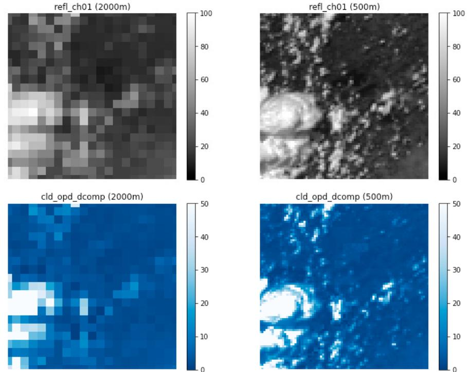
Example of super resolution cloud products identifying small scale features that effect solar radiation. Visible reflectance measured from the GOES-16 satellite (top panels) show a cloud 'self-shadowing' effect in the 500 m retrievals (right panels) not seen in the 2000 m retrievals (left panels). This effect can be seen in the retrieved cloud optical depth (bottom panels), which will impact solar radiation fields estimated at the surface. This scene is over Madison, Wisconsin.
