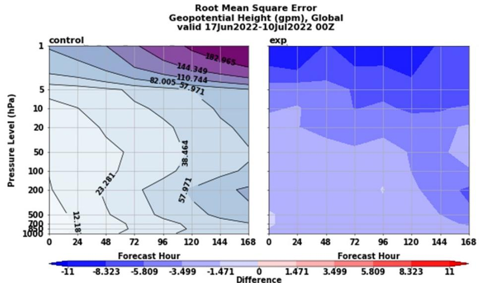
The left panel indicates the geopotential height forecast error growth within the model out to 168 hours of the control. The right panel is the *change* in geopotential height error growth when using the new profile selection criteria. The varying shades of blue indicate improvements (less error) in the geopotential height forecast when using the new profile selection scheme.
