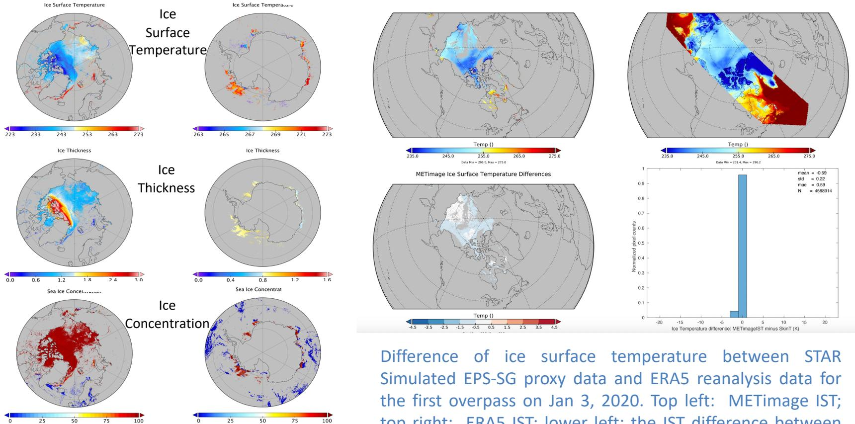
Daily clear sky composite ice products from EPS-SG METImage proxy data. The ice surface temperature (K), ice thickness (m) and ice concentration (%) from the top to the bottom sequentially on January 3, 2020 for the Arctic Ocean (left column) and the Antarctic Ocean (right column).
