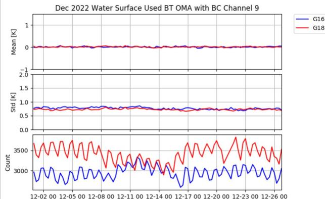
CSR minus GFS Analysis brightness temperature mean, standard deviation, and data count for ABI Channel 9 with the VarBC bias correction in GSI for used water surface observations.
