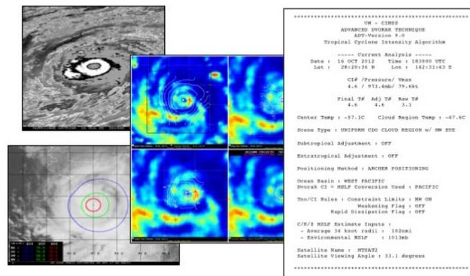
Example of ADT output products derived from image analysis including TC center location, 2D wind radii, MW structure, and intensity estimates
