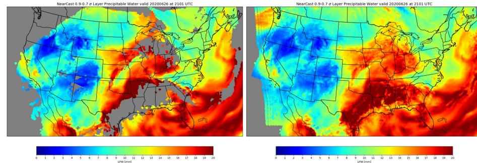
0.9-0.7 sigma layer precipitable water valid 2101 UTC 26 June 2020 using GOES-only (left) and GOES+MiRS (right) profiles for heavy rain event south central WI. MiRS improving product utility and consistency by filling most GOES data gaps
