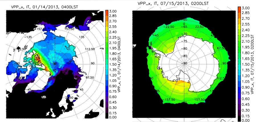
The Arctic (left) and Antarctic (right) sea ice thickness retrieved with VIIRS data on January 15, 2013 (Arctic winter) and July 15, 2013 (Antarctic winter), respectively.
