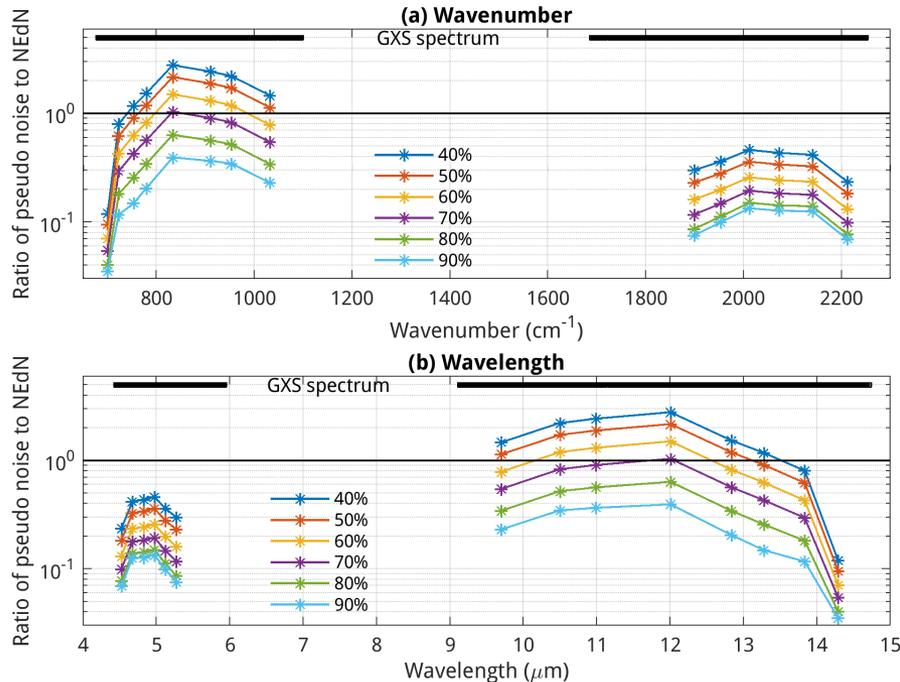
The ratio of pseudo noise to the instrument noise equivalent radiance differential (NEdN) for different EE values. The EE numbers are determined based on  $680 \text{ cm}^{-1}$
