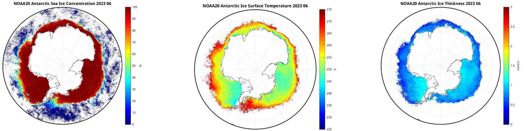
Ice Concentration (left), Ice surface temperature (middle), and ice thickness (right) from NOAA-20 VIIRS monthly composite data under clear sky conditions.
