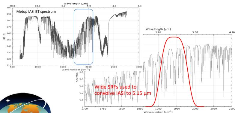
IASI BT spectrum and 4.8–5.9  $\mu\text{m}$  spectral range with 5.15  $\mu\text{m}$  SRFs overlaid in red.
