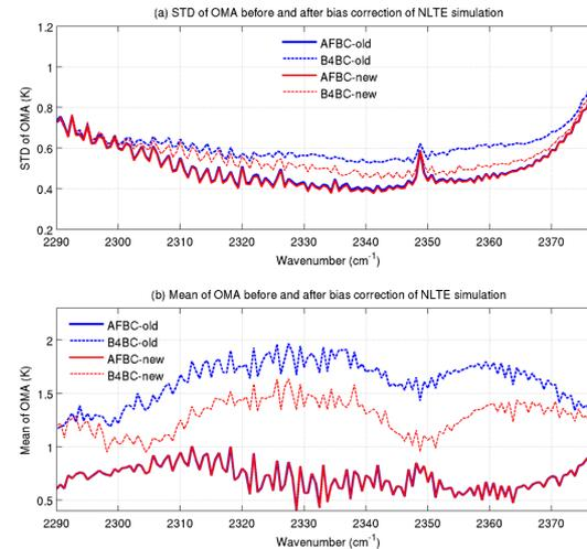
Daytime observation – analysis (O-) (before and after bias correction of NLTE simulated from CRTM. Dashed lines indicate before bias correction (B4BC) and solid lines are for after bias correction (AFBC). Two sets of CRTM coefficients are used here. (a) Standard deviation and (b) mean.
