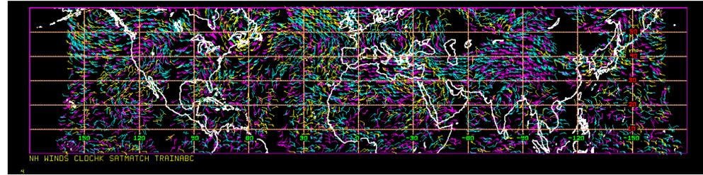
Scenario: Nine polar-orbiting satellites flying as 3-satellite trains each equipped with a hyperspectral IR sounder. Equator crossing times of 0530, 0930, 1330 local time. The figure depicts the AMVs derived from the ECO1280 in a three-hour time window covering latitudes from equator to 60° N. Color coded by height: Yellow below 700 hPa; cyan 400-700 hPa; magenta above 400 hPa.
