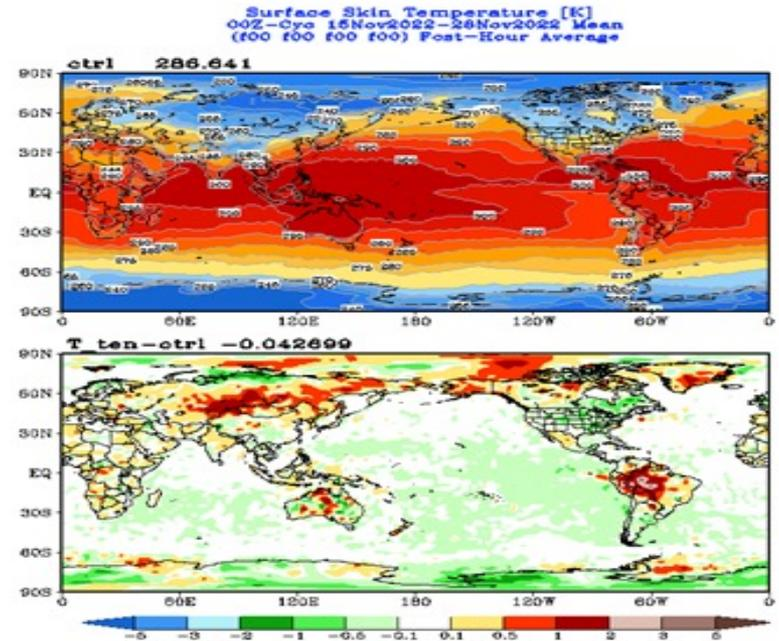
Top panel is average analysis skin temperature from 15 Nov – 29 Nov 2022 for the control (ctrl). The bottom panel is the analysis difference between assimilating the temperature radiance tendency ( $T_{ten} - ctrl$ ).
