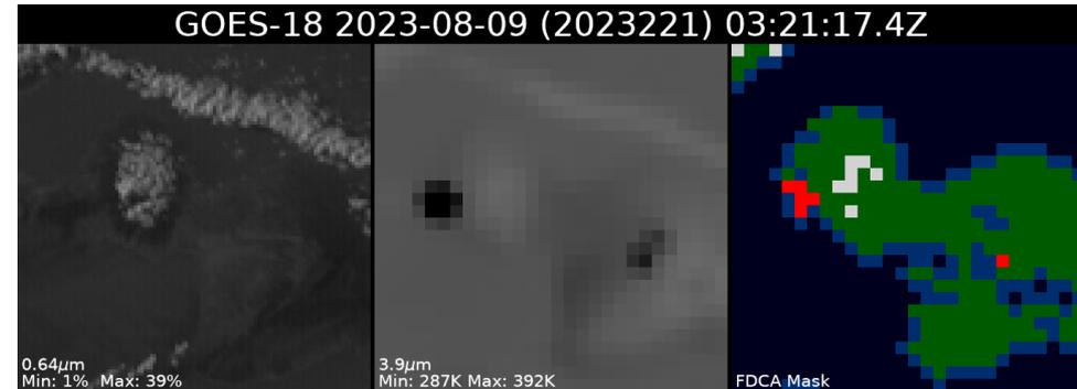
Left to right, GOES-18 visible and 3.9 µm (fires are dark) raw data and the FDCA mask (red is detected fires) for Maui on 9 August 2023.
