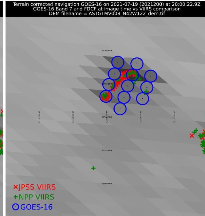
GOES-16 3.9  $\mu\text{m}$  imagery of a fire in Oregon on 19 July 2021 (left: standard navigation, right: terrain corrected). Users at the Satellite Analysis Branch had noted the offset between VIIRS fire detections (red and green markers) and the FDC product (blue circles). Terrain correction of the FDC detections and the underlying GOES data showed excellent agreement between the two instruments. The temporal difference between the scans was less than 5 minutes.
