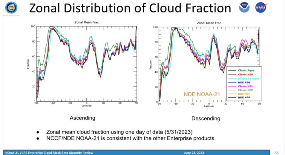
Comparison of the zonal cloud fraction for NOAA-21 as compared with other processing systems done for the NOAA-21 ECM Beta review, showing that the ops code performs as expected
