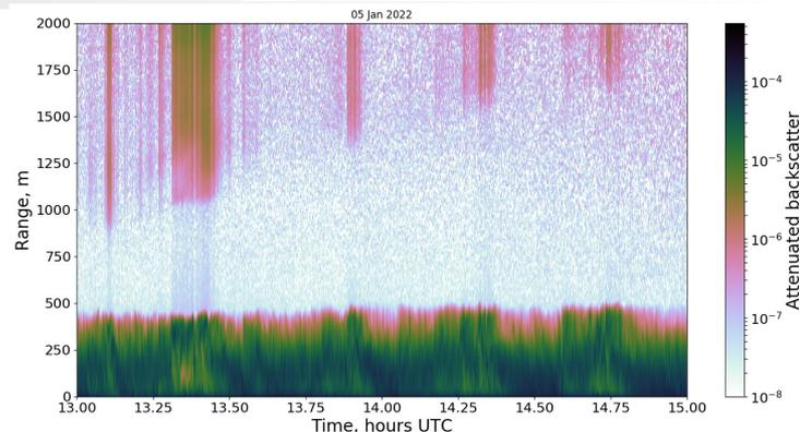
Ceilometer-observed lidar backscatter profiles for blowing snow near the surface with cloud aloft from our field site near Emerado, North Dakota
