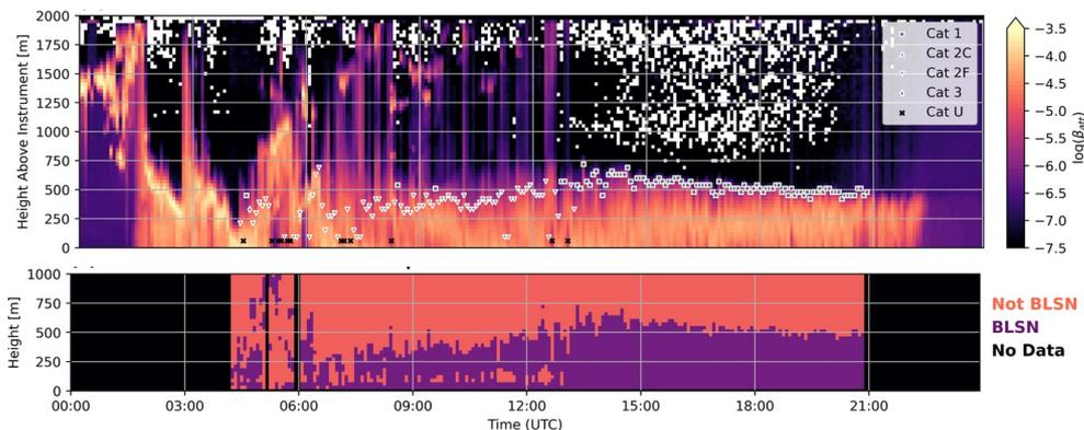
Machine-learning algorithm determines (top) snowfall categories and (bottom) extent of blowing snow from ceilometer backscatter profiles.
