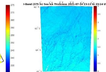
Examples of the highest resolution (via I-band, 375-m) of ice concentration (left), ice temperature (middle) and ice thickness (right) for various cases from NOAA-20 with time stamps given above the image. Note that data only available under clear sky condition determined by VIIRS CM.
