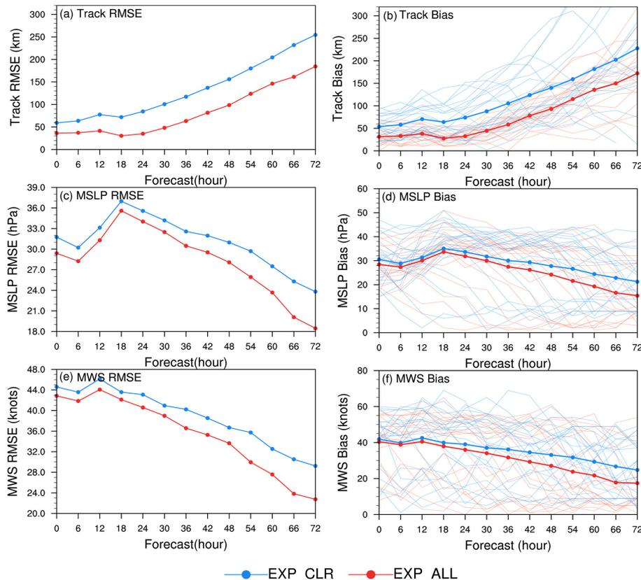
The forecast (left) RMSE and (right) bias of track, minimum sea level pressure (MSLP), and maximum wind speed (MWS) of Hurricane Irma as a function of forecast time. The light blue and light red lines in (b, d, and f) are the forecast biases for each initiating forecast time.
