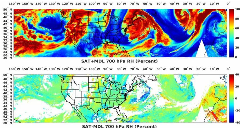
Satellite sounding/model 700-hPa relative humidity (top) and satellite/model difference (bottom).
