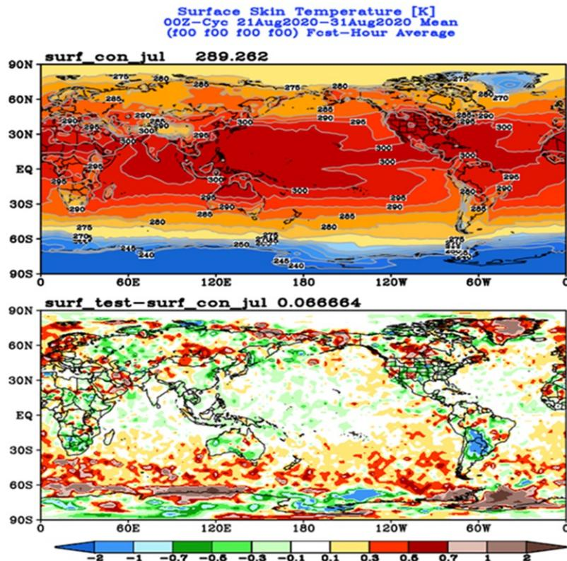
Surface skin temperature from the experiment consistent with operations (surf\_con, top) and the difference generated from using the new infrared sea surface emissivity model (surf\_test – surf\_con, bottom). The greatest differences are in the cold-water regions where temperatures are increased by up to 0.6K. This is consistent with the expected theoretical temperature differences.
