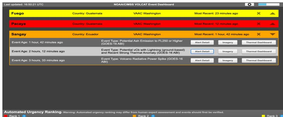
Screenshot of the VOLCAT Event Dashboard demonstrating the incorporation of lightning data in VOLCAT. In this example, VOLCAT issued a vCb alert (due to rapid cloud growth) with lightning present from a ground-based network (ENI).
