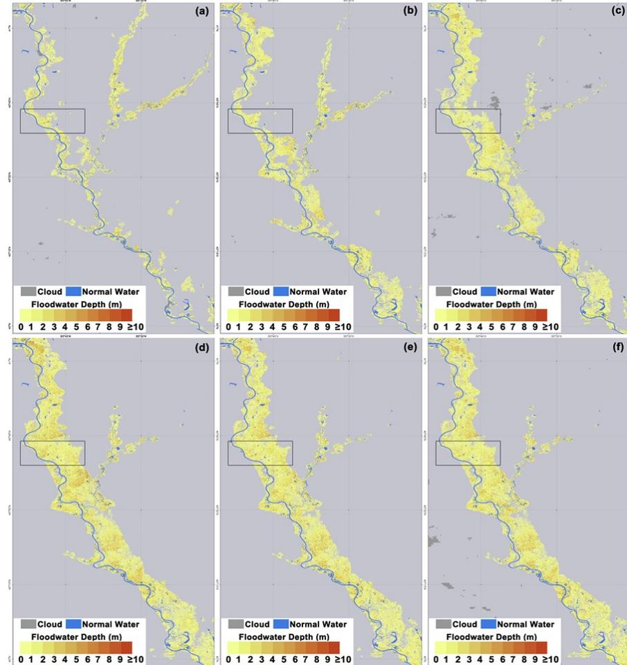
VIIRS downscaled 30-m floodwater depth along the Missouri River 2019: (a) 3/15, (b) 3/16, (c) 3/18, (d) 3/20, (e) 3/21 and (f) 3/22.
