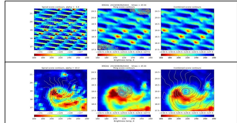
Example of incorrect microwave data reading and plotting issue at CWB (top) and corrected display after CIMSS code fix delivery
