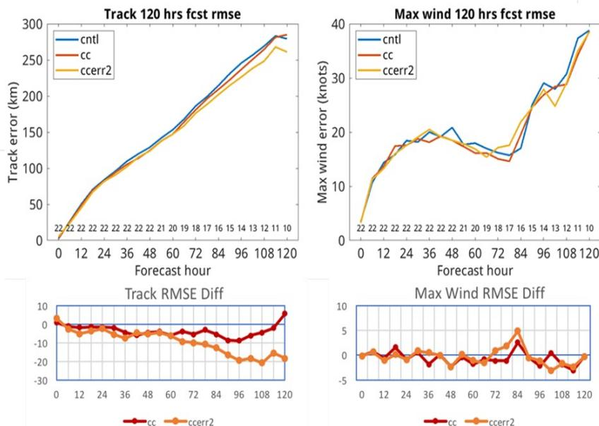
The RMSE of track (upper left) and maximum wind speed (upper right) forecasts for hurricane Irma in 2017 from three different experiments. The lower panels show the RMSE difference from the control for the track (lower left) and the maximum wind speed (lower right).
