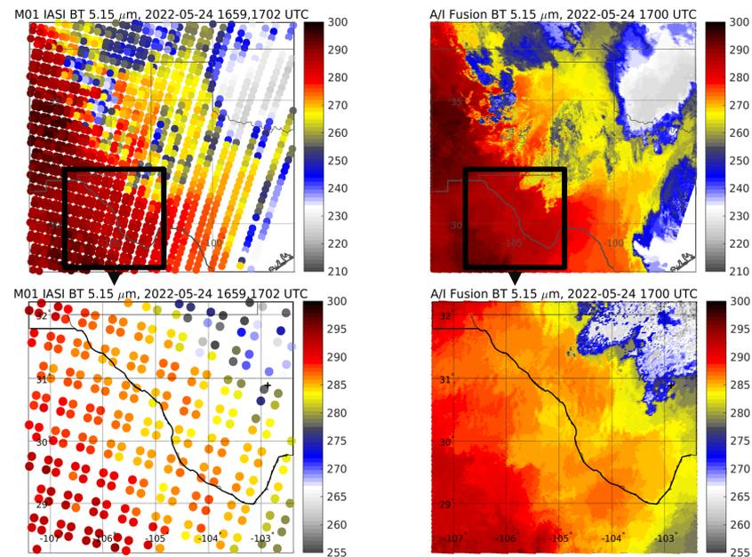
IASI (left) and ABI/IASI Fusion (right) 5.15  $\mu\text{m}$  Brightness Temperatures [K] over the New Mexico/Texas border on 24 May 2022.
