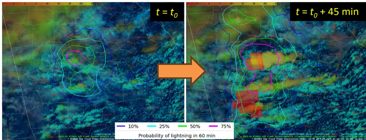
LightningCast probabilities (contours) in Georgia. Background is GOES-16 day cloud phase distinction RGB. Orange-to-yellow foreground pixels are Geostationary Lightning Mapper flashes.
