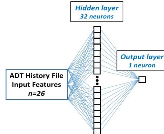
Schematic diagram of the AiDT Neural Network model, consisting of 26 input parameters (from ADT analysis) and an output wind speed estimate
