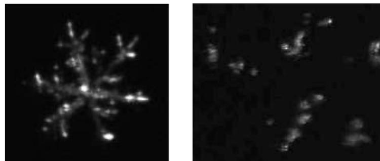
Distinct particle characteristics during (left) falling snow with pristine particles versus (right) blowing snow with fractured and rounded particles from imager observations.
