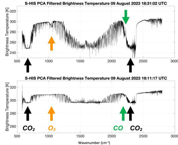
Examples of S-HIS upwelling atmospheric spectra for two single footprint observations during the August 9, 2023, flight. The top panel corresponds to a high-altitude approach over Pennsylvania and the bottom panel corresponds to a low-level flight leg over New Jersey.
