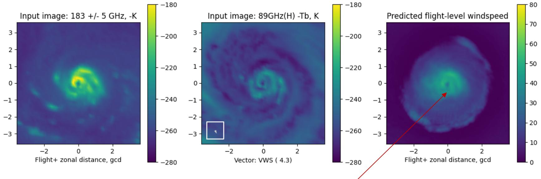
The model resolves small eyes and a double eyewall, as revealed in the ATMS imagery
