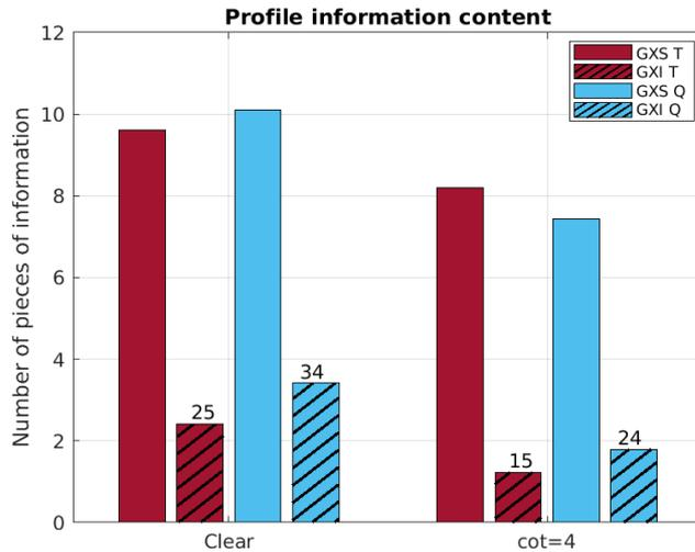
The information content of GXS and GXI for temperature and moisture in both clear and cloudy conditions. The numbers on top of the bars indicates the percentage of information content from GXI compared to GXS. The cloud has a cloud optical thickness of 4 and cloud top pressure at 300 hPa. The tropical atmosphere profile is used.
