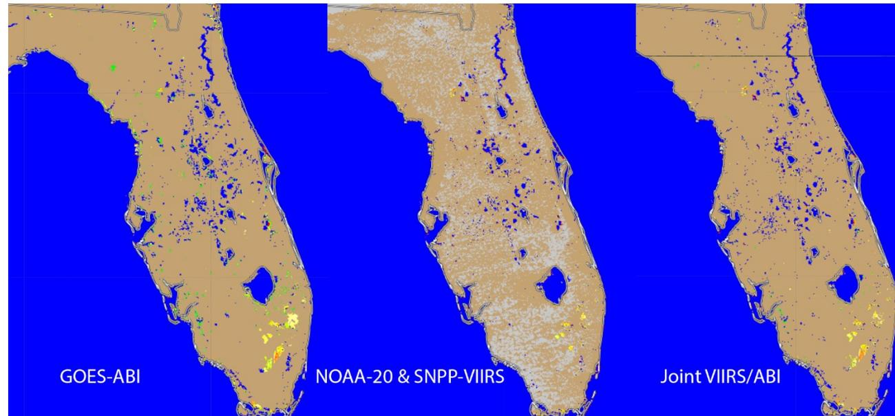
Example ABI (left), VIIRS (center), and Joint flood product (right) over Florida from March 15, 2020. This case does not contain significant flooding but does illustrate how the cloud cover (grey) can be reduced by using a time series of geostationary imagery.
