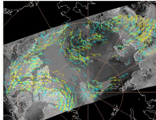
Simulated 10.69  $\mu\text{m}$  IR METImage data; 3 Jan 2000 at 0217 UTC. Raw winds (cyan); quality controlled (yellow).
