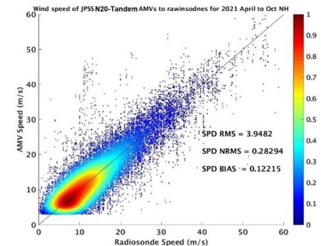
April through October Arctic VIIRS AMVs compared to rawinsondes, for NOAA-20 single-satellite (left) and S-NPP/NOAA-20 tandem (right). Density scatter plot of VIIRS AMVs vs rawinsonde wind speed.
