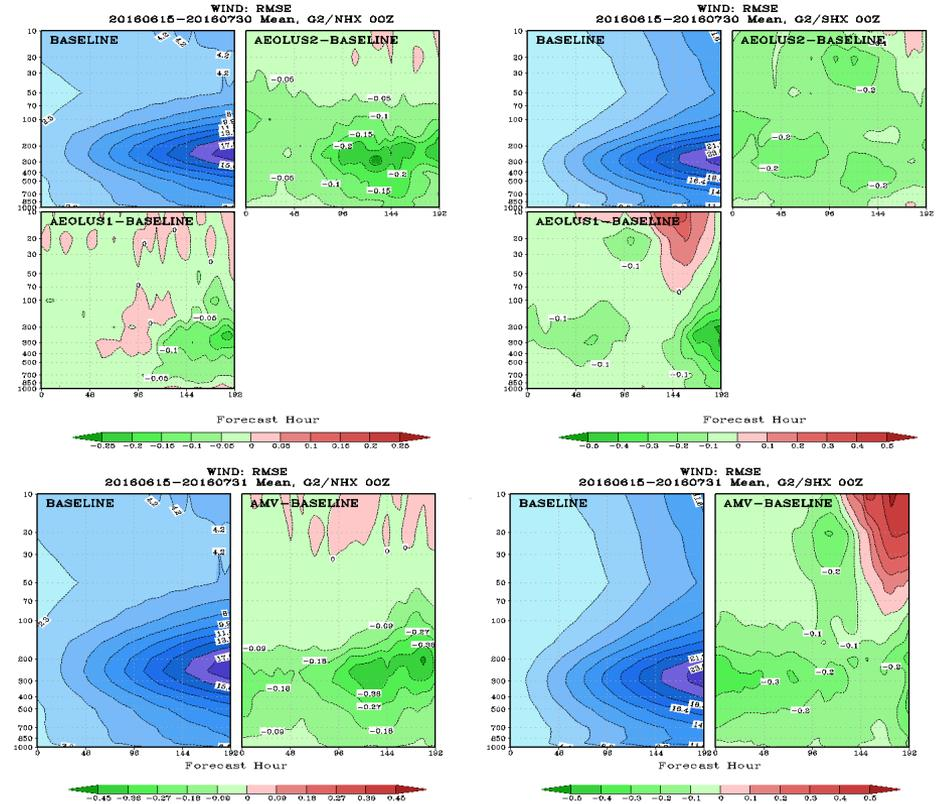
Forecast wind field root-mean-square (RMS) cross section for Northern (left) and Southern Hemisphere.(right). (Top) Aeolus1 assimilates wind observations from the current Aeolus configuration. Aeolus2 assimilates wind observations from Aeolus follow-on which has a higher laser power. (Bottom) AMV assimilates passive winds retrieved at 8 pressure levels from 3 polar orbiters.
