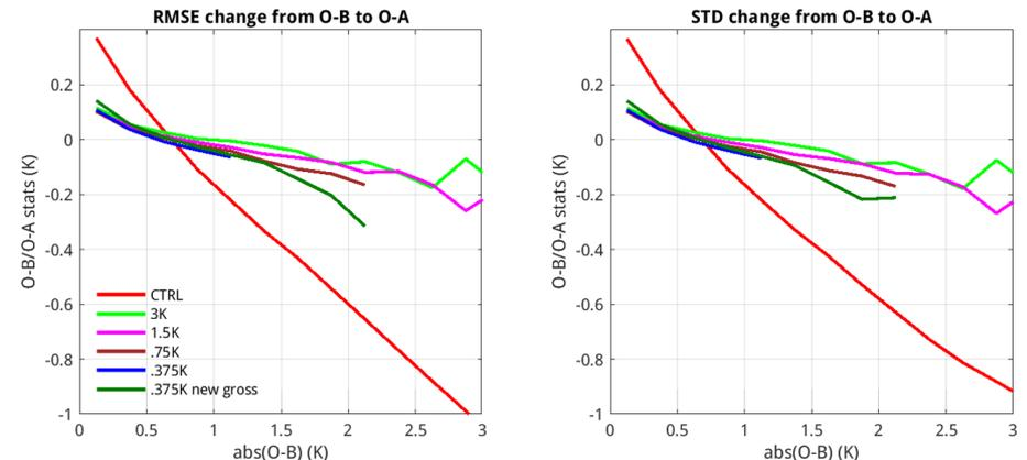
Change in observation minus background (O-B) and observation minus analysis (O-A) (left) root mean square error (RMSE) and (right) standard deviation (STD) for ABI band 8. Control (CTRL) is the operational setup. Remaining experiments assimilate tendency observations with observational errors of 3, 1.5, 0.75 and 0.375K. 0.375K new gross uses prescribed values estimated from the histograms of radiance tendency measurements for gross check.
