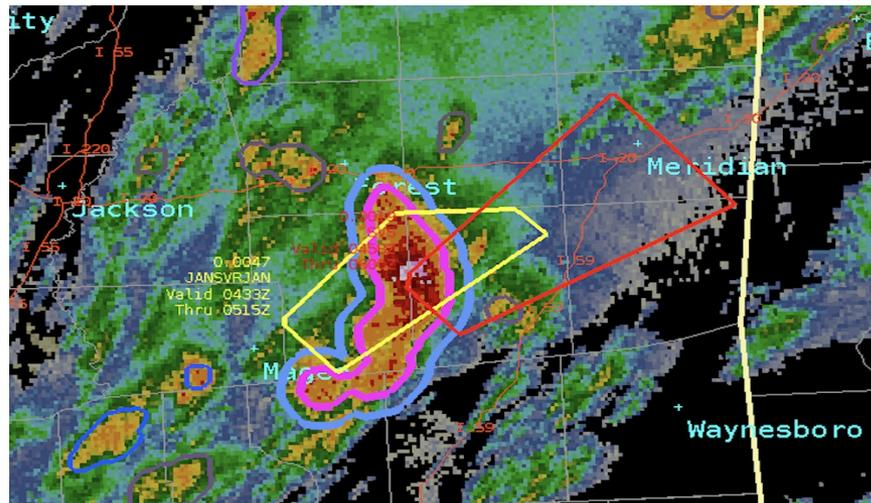
ProbSevere storm-object contours for a tornado-warned storm in Mississippi. The pink contour signifies  $\geq 85\%$  probability of any severe, and the light blue contour represents 40% probability of tornado.
