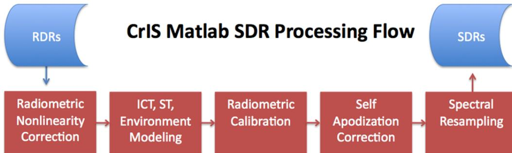
**Figure 14.6.2.** CrIS Sensor Checkout Data Analysis Flow.
