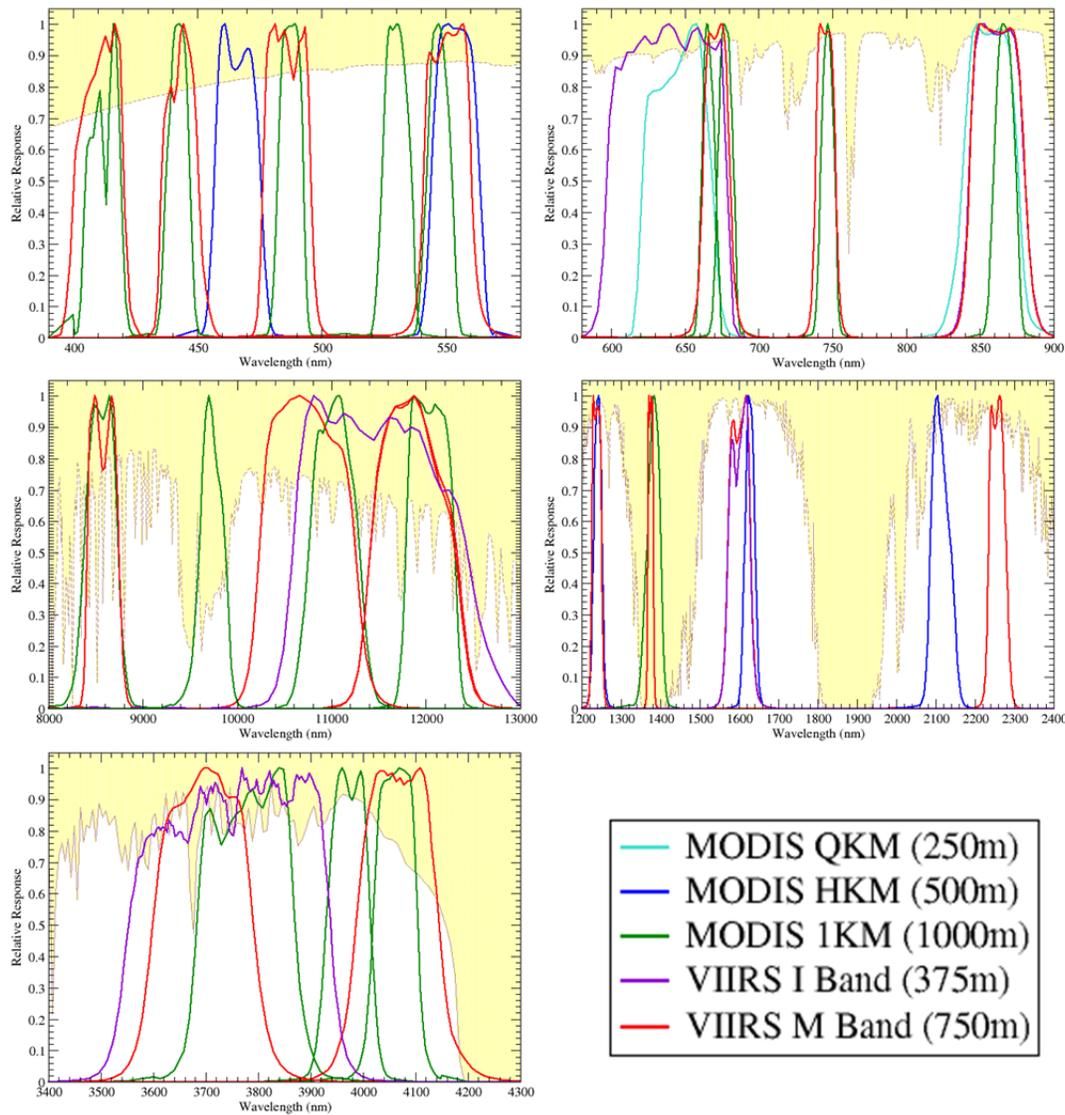
**Figure 14.2.1.** Government team “best” sensor level in-band Relative Spectral Response (RSR) for VIIRS Flight 1 instrument, shown with Aqua MODIS RSR. The government team independently derived VIIRS RSR to support and verify industry RSR and specification compliance, as well as to identify value added measures to improve the RSR information content. Color coded legend applies to all panels. Model based atmospheric extinction is represented by the yellow background of each panel.
