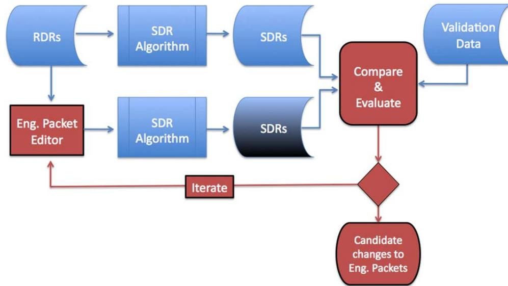
**Figure 14.6.1.** CrIS Sensor Checkout Data Analysis Flow.
