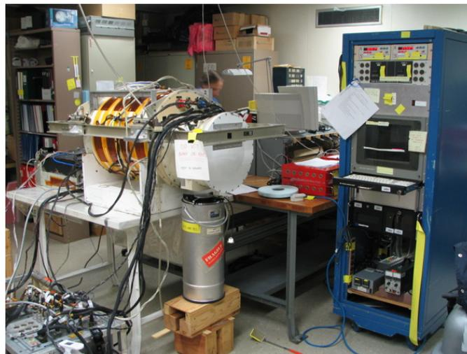
**Figure 17.4.5:** NAST-I External Ice Bath Blackbody reference source test configuration, used both before and after the JAIVEx field campaign.
