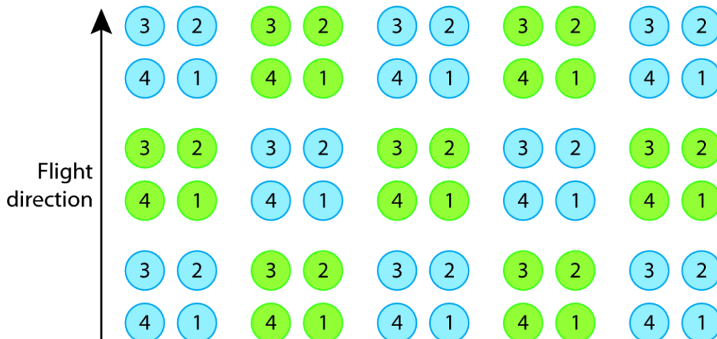
Figure 1: Simplified schematic of the IASI scan pattern, showing the pixel numbering for the four pixels within an AMSU-A field of view, relative to the flight direction. The colour coding corresponds to the alternating direction of the movement of IASI's corner cube mirror.
