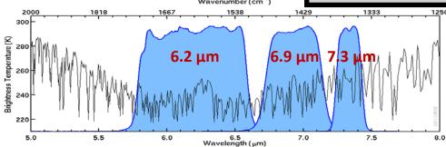
Spectral response functions for the three ABI Water Vapor Bands, along with clear-sky top-of-atmosphere brightness temperature for a USA Standard Atmosphere. Cooling due to water vapor is strongest in the 6.2 µm channel
