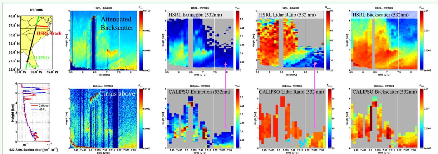
Qualitatively good agreement seen between CALIOP level 2 aerosol profile products and HSRL (averaged to 40km). CALIOP identifies the change in lidar ratio but misidentifies the type near 7.53 UTC, causing higher retrieved extinctions than measured by HSRL.
