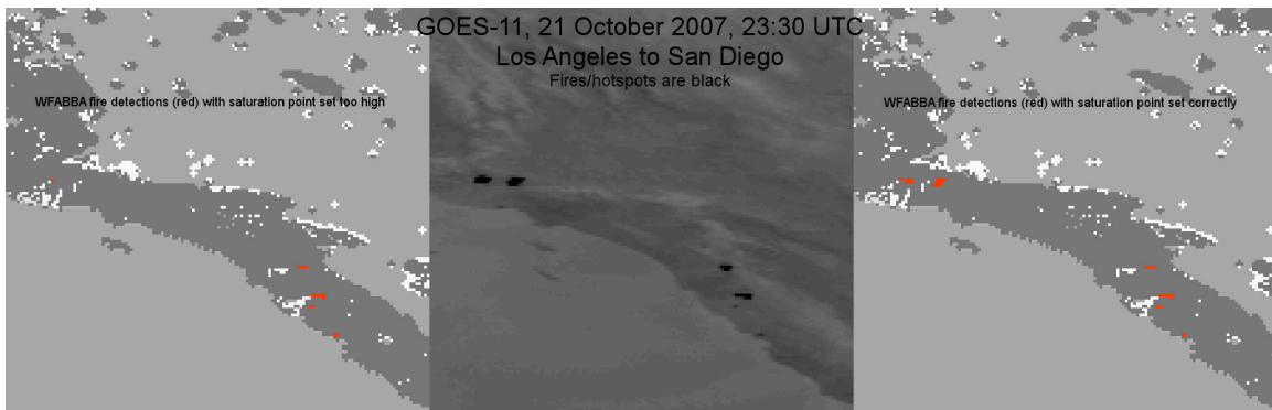
Figure 7. Complex of major fires, GOES-11 3.9 \mu\text{m} band, 21 October 2007 (center); Original WFABBA metadata mask, fires in red (left); WFABBA metadata mask with adjusted saturation point, fires in red (right)
