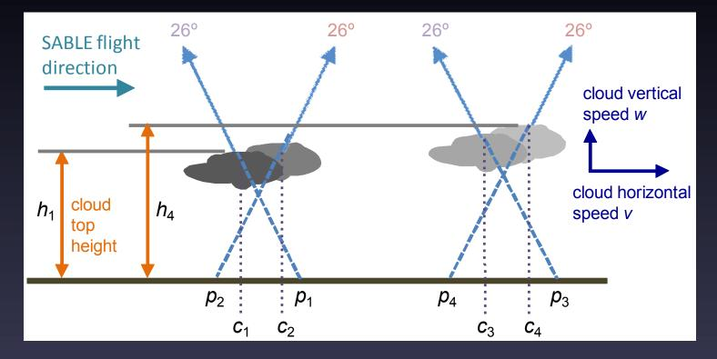
Along-track motion and height parallax are *independent* Sensitive to vertical motion
