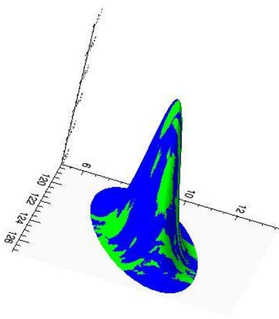
Figure 4. ATMS 5.2° fov at the 99% power level, with DEM warped over the relative antenna power.
