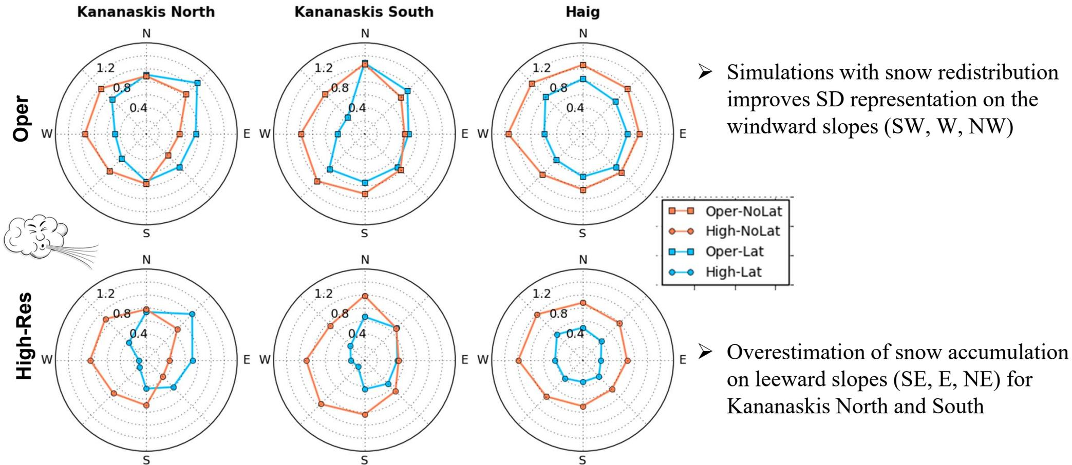
➤ Simulations with snow redistribution improves SD representation on the windward slopes (SW, W, NW)
