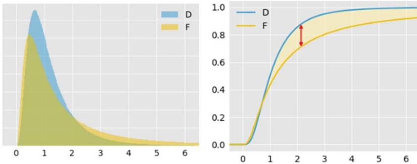
**Wasserstein distance** between cumulative distribution functions:
