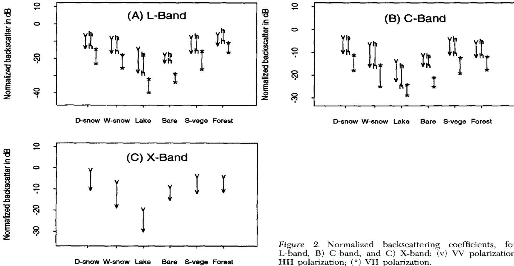
Figure 2. Normalized backscattering coefficients, for A) L-band, B) C-band, and C) X-band: (v) VV polarization; (h) HH polarization; (\*) VH polarization.
