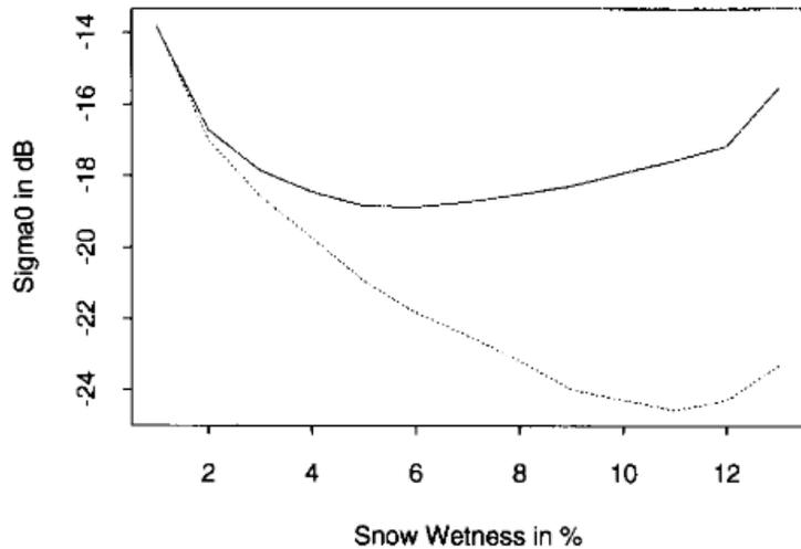
Relation between simulated C-band backscatter signal at polarization VV and snow wetness and snow/air interface roughness
