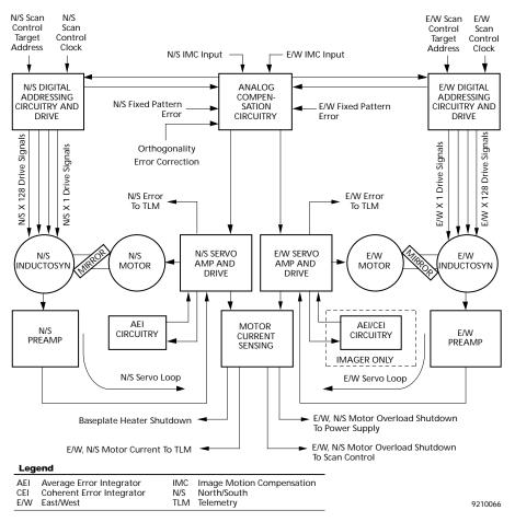
is developed for the precise control of position in response to a system-level control processor.
