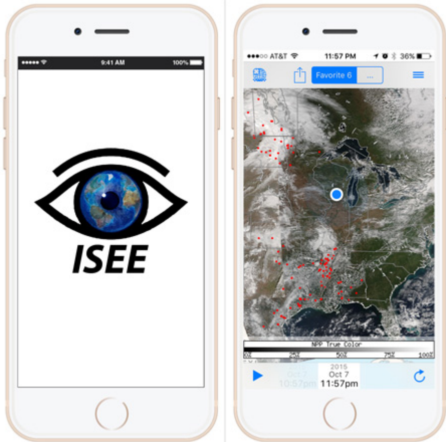
Figure 70. ISEE iOS Prototype App display of daily S-NPP VIIRS True Color Composite with VIIRS Satellite Detected Fire Locations (newest available) from VIIRS Active Fire team at University of Maryland ( http://viirsfire.geog.umd.edu/ ). This is an actual screenshot from an iPhone 5s.
