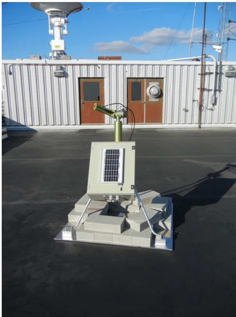
Figure 15.1. Photo of CIMEL Sun Photometer at UW-Madison Engineering Research Building, 1500 Engineering Drive Madison, WI 53706.
