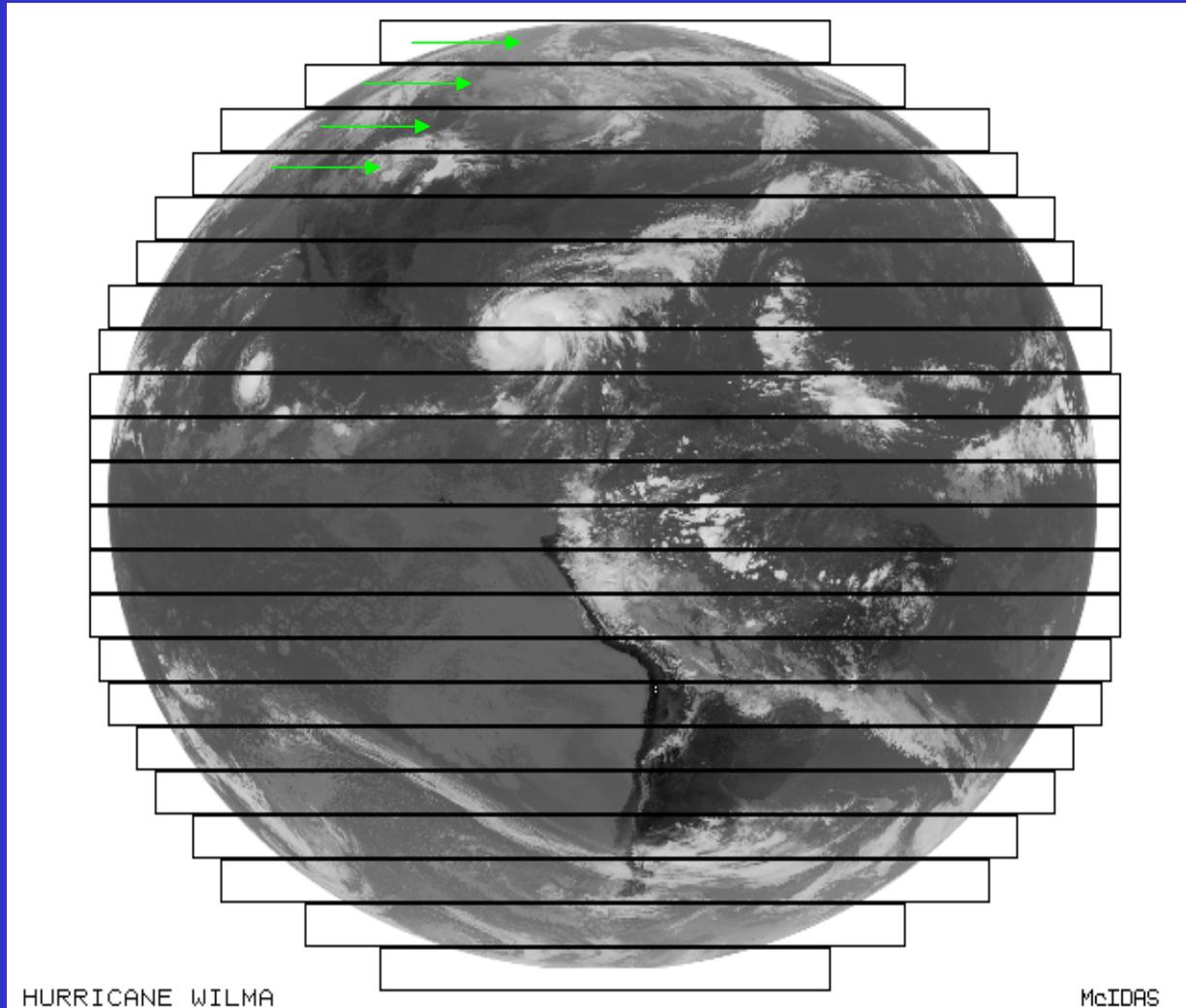
The ABI instrument can scan west-to-east OR east-to-west, the alternating pattern 'swath-to-swath' of the GOES-I/N series will not be continued. 9
