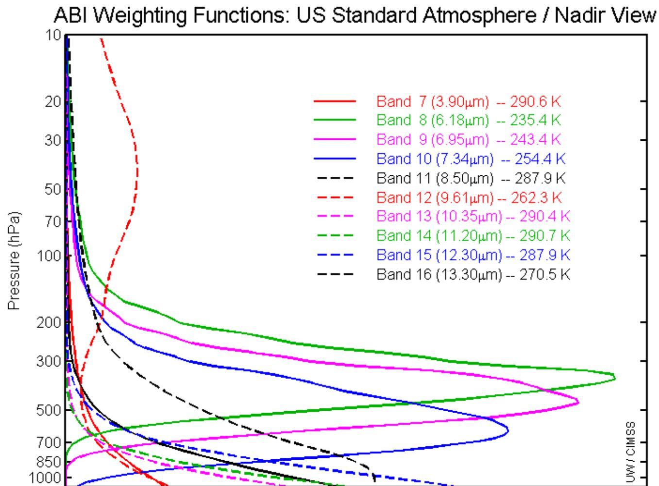
ABI has 1 CO<sub>2</sub> band, so upper-level temperature will be degraded compared to the current sounder
