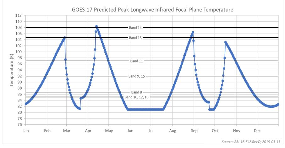
This plot shows daily maximum temperature of the ABI focal plane module. These maximums occur at night. The higher the temperature, the more saturated imagery becomes. Where the temperature rises to approach a black line for each band, marginal saturation may be observed in imagery. Where the temperature curve exceeds a black line for each band, the imagery may begin to saturate so much that it becomes unusable.
