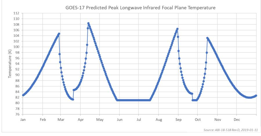
This plot shows daily maximum temperature of the ABI focal plane module. These maximums occur at night. The higher the temperature, the more saturated imagery becomes.
