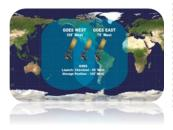
There are two GOES currently orbiting and viewing the continental US. One is called GOES-East; the other is called GOES-West. In addition, there is an onorbit spare, which can be used in the event of an emergency or malfunction of the East and West satellites.
