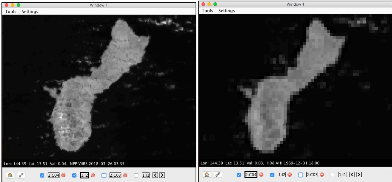
Figure 2: HYDRA display of VIIRS I-Band 2 (.86 \mu\text{m} ) 375 m reflectances in the left panel, and AHI “Veggie” Band 4 (.86 \mu\text{m} ) 1 km reflectances in the right panel from datasets observed over Guam at 03:35 UTC and 03:40 UTC respectively.
