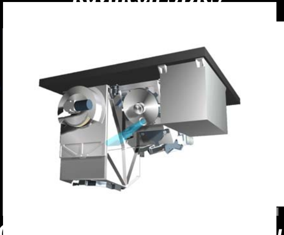
Visible/IR Imaging Radiometer Suite (VIIRS) Raytheon SBRS
