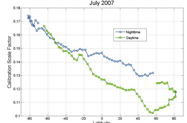
The one major problem, as shown by the plots above and to the left, is that there appears to be a pronounced latitudinal structure to the calibration scale factor. This is believed to be an instrument artifact similar in nature to the thermally induced beam steering problem that effects the
