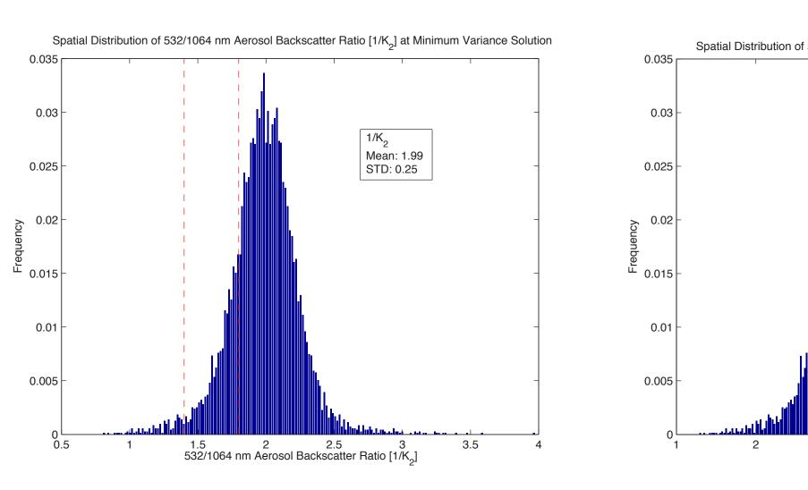
• At left is the spatial distribution of the aerosol backscatter spectral ratio (532 to 1064 nm). At right is the spatial distribution of the aerosol extinction spectral ratio.
