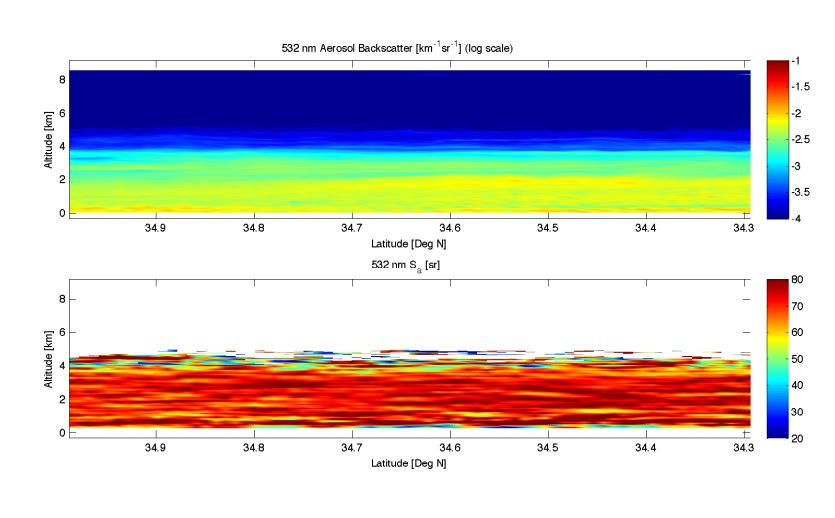
• At left, the HSRL flight track with the region of interest marked in red • At right, the 532 nm aerosol backscatter and S<sub>2</sub> measured by HSRL • The spatial consistency of the S<sub>v</sub> verifies the constraint necessary for E-CRAM (equation 1)
